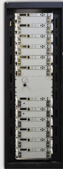
6.6W C-Band or X-Band Rackmount SSPA GaN Based - SapphireBlu™ Series
